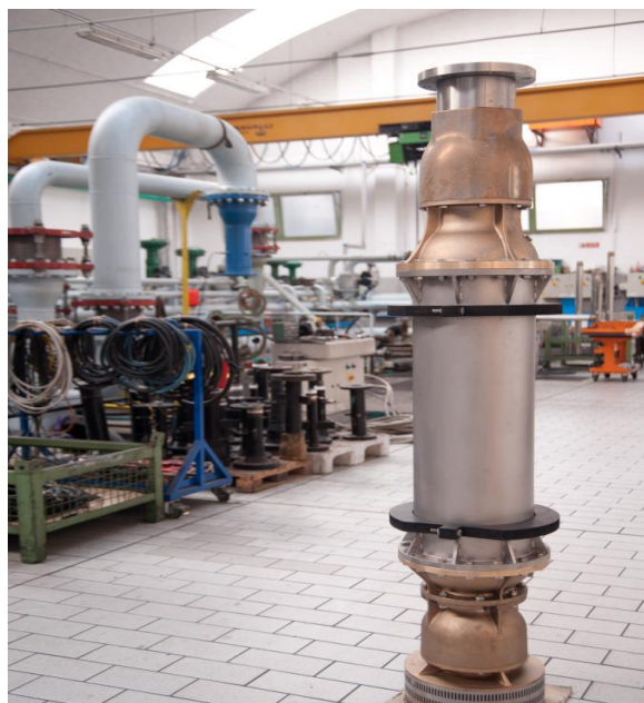
Fig. 3 SM: ballast pump. On the background: testing room in the headquarter
