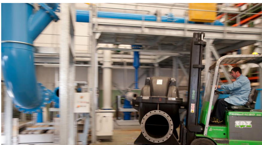
Fig. 5 Split casing SKD and in the background the testing room in submersible motors plant
